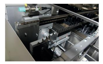
For short process times, a pure inline process can also be used. In this case, a pin chain can provide the edge support for the products in the furnace, equivalent to holding the specimens in the system. The advantage is that heat can be introduced unhindered from above as well as from below. With pin chain transport, the transport width can also be variably adjusted so that the system can be adapted to different product widths.
