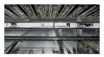
In the combination heating process, heat is transferred by infrared radiation, which can be supported by central convection heating. All heating chambers are equipped with powerful IR radiators. This enables a faster and more efficient drying process. With the additional convection, the volume flow can be preset. To reduce residue and to protect against soiling and for easier cleaning, all IR emitters in the heating base can be optionally fitted with glass covers.
