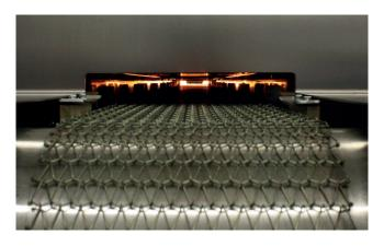
In the case of thin substrates, such as the membrane, full-surface support on a conveyor belt is recommended. Depending on the requirements of the product, a braided or woven belt made of different materials can be selected here.
