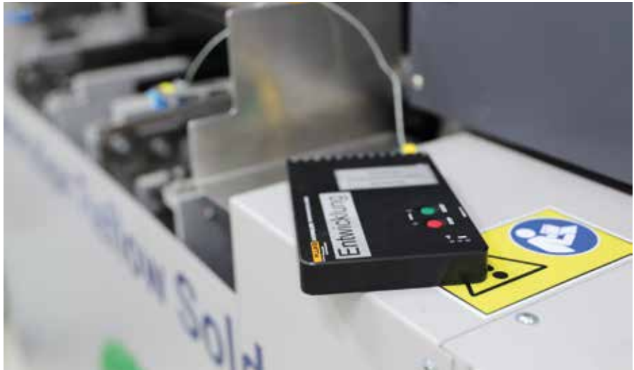
A temperature data logger can be used to monitor the temperatures of various applications in real time.
